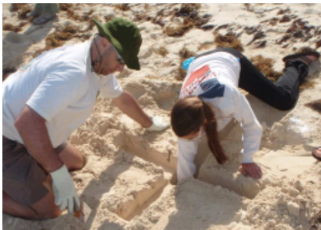
Figure 6. Mold for REDs hand dug in beach sand.
