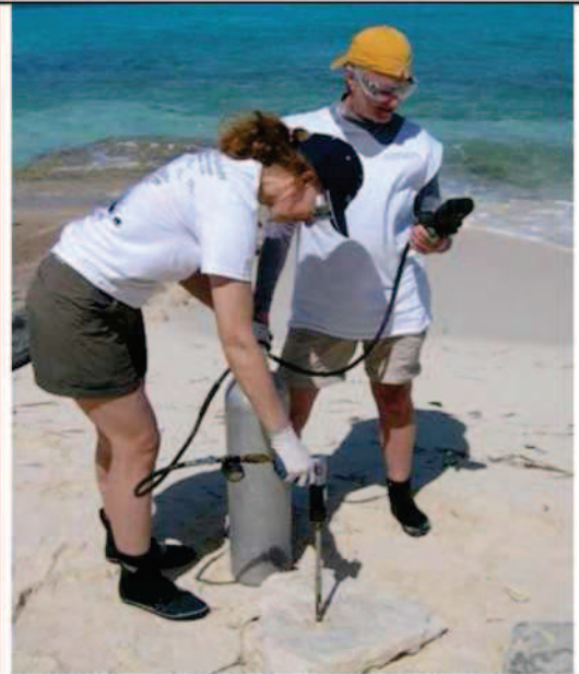
Figure 2 – SCUBA regulator and hoses modified to power air drill with an air tank.
