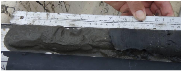
Figure 2. Core 21 from Bay Champagne, taken after Hurricanes Gustav and Ike, contains a 17 cm-thick layer of unconsolidated sandy clay at the top that represents a storm deposit caused by these hurricanes (From Liu et al., 2011).
