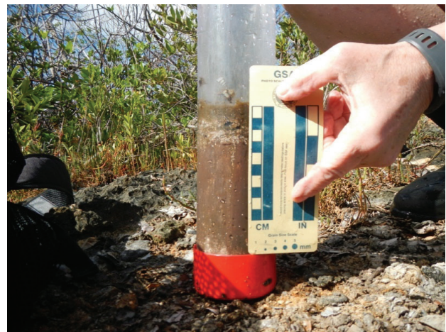
Figure 5. Oyster Pond southern conduit core taken in 2016. Shell-hash layer on bottom not visible due to lower core cap. Upper shell hash is likely hurricane deposit.
