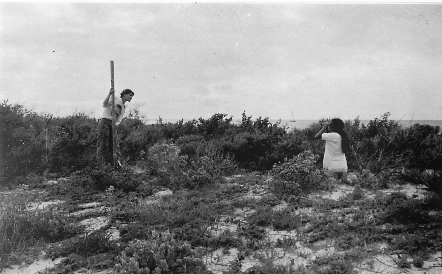
Figure 3: Topographic surveying method: Kat Herchenreder on the left holding a meter tape "survey rod", and Meera Sundaram on the right using a hand-held level.
