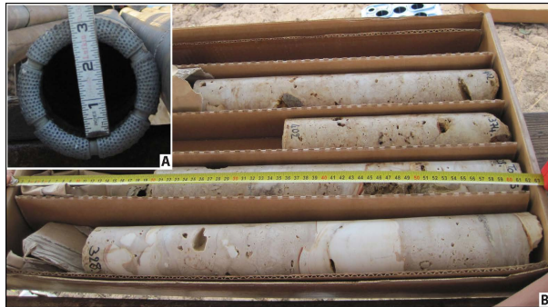
Figure 6. 10 cm-diameter drill bit with 6.3 cm-diameter core pieces stored in a cardboard box. A) Surface-set diamond coring bit and HQ core barrels, scale in inches. B) Core pieces showing the karstified Mayaguana Formation between 2.80 m below the island surface (mbis) and 4.42 mbis.
