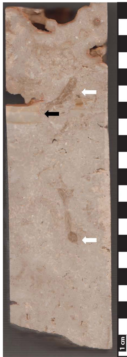
Figure 7. View of the retrieved basal core piece from 43.07 mbis to 43.30 mbis. White arrows indicate rhizoliths; black arrow shows the geopetal infill of a dissolution void.
