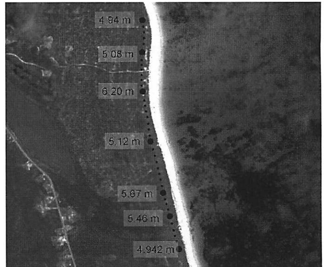
Figure 4. Aerial image of East Beach showing the approximate position of the debris strand line and selected elevation values (Image ©2010 Digital Globe and © 2009 Google).
