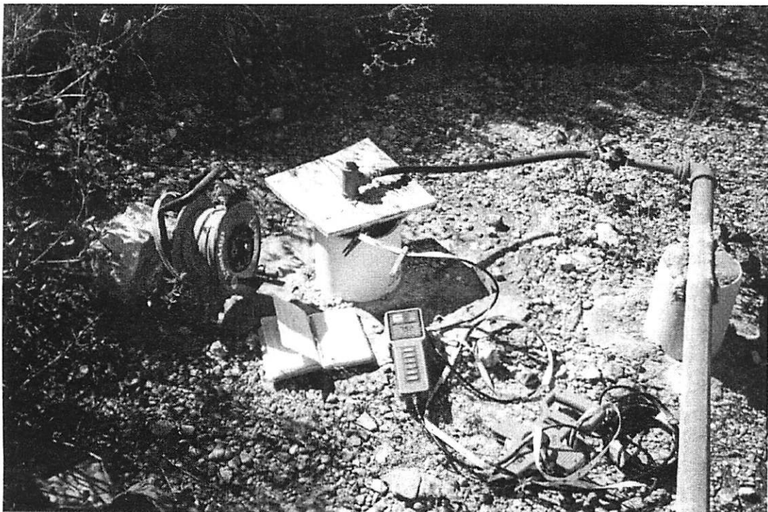
Figure 8: Well measuring set-up. The water level indicator is to the left of the well and the conductivity meter (with tape measure attached) is in the foreground. The probe is down the well.
