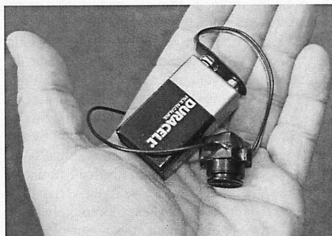
Figure 2. Supercircuits's "nanobug" wireless ATV video camera with attached transmitter. Wire at left is the antenna.
