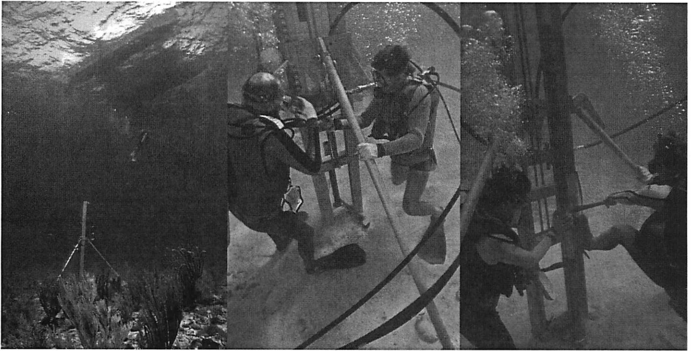
Figure 2. Underwater photographs of the SCARID drilling system A (left). Drill on the bottom at site LBN-02 off eastern St. Croix. The support barge is visible at the top of the photo. Hoses deliver hydraulic power and water from the surface. Water depth is 13 meters. B (middle). Diver lowering the drill assembly using the hand crank. Strong tactile feedback through the drive assembly allows the operator to “feel” the character of the substrate being cored. Changes in drilling character are referenced to the scale on the left side of the drill and are recorded on a lexan slate. C (right). Divers adding a section of drill pipe after recovering the previous 150 cm of core. Core is trapped in a separate inner barrel that can be recovered remotely without removing the drill string. Core is removed from the inner core barrel on the surface and referenced to the drilling notes kept by the operators on the bottom.
